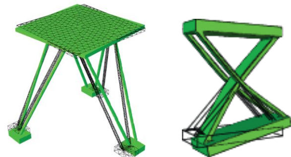
Conversion of beam model into Pseudo-Rigid-Body model
